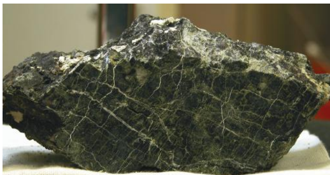
Samples of serpentinized and carbonated peridotite from different field sites have helped DCO scientists understand the role of carbon during serpentinization (this example is from the Atlantis Massif and is about 20 centimeters long).
